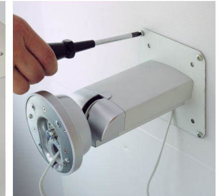
Mount the Hinge Device on the wall
