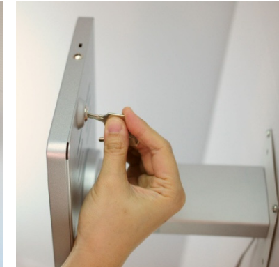
Lock the top cover with hex key or/and the CAM-lock in the back of enclosure
