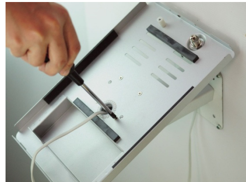
Mount the Enclosure to Hinge Device
