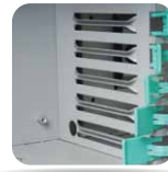
Tool-less card retainers
