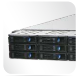
Front accessible modular HDD cage (12 x 3.5 HDD)
